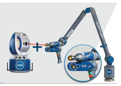
The FARO® Super 6DoF TrackArm is the most versatile portable 3D measurement system that brings together the latest advancements in FARO's 3D measurement technology to deliver a solution that allows flexibility, ease of use and un-compromised accuracy for your most demanding 3D measurement needs. The system combines the long-range and high accuracy capabilities of FARO's Laser Tracker with the flexibility, detail, and consistency of the FaroArm® and/or ScanArm.
